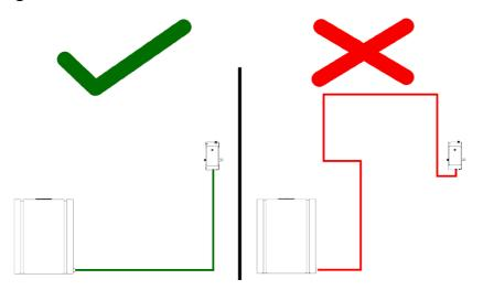
Recommended installation is shown in the picture below. Cabinet placed close to the hose reel with a maximum distance of 25 meters. Directly placed underneath are two 25-liter chemical containers placed in our stainless-steel wall hangers.
