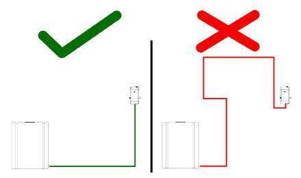
Recommended installation is shown in the picture below. Cabinet placed close to the hose reel with a maximum distance of 25 meters. Directly placed underneath are two 25-liter chemical containers placed in our stainless-steel wall hangers.
